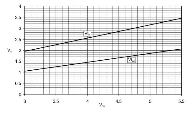
Figure 27: Schmitt Trigger typical input voltage thresholds vs. V<sub>DD</sub>
