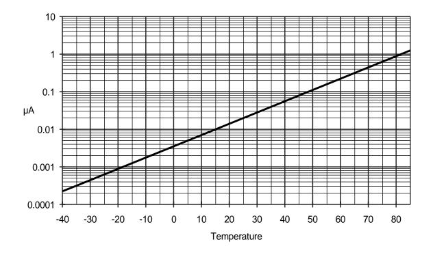
Figure 28: Typical 'Zero-Power' I<sub>DD</sub> vs. Temperature (V<sub>DD</sub> = 5.0V)
