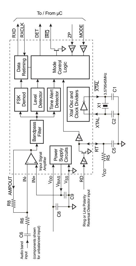
Figure 1: Block Diagram
