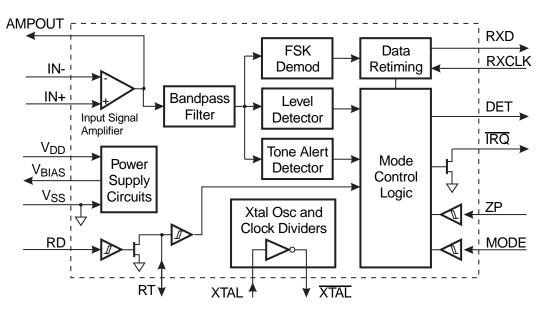
The MX602 is a low power CMOS device used for the reception of physical layer signals in Bellcore's Calling Identity Delivery (CID) and Calling Identity on Call Waiting (CIDCW) systems, British Telecom Calling Line Identification Service (CLIP), the Cable Communications Association's Caller Display Services (CDS), and similar evolving services.
