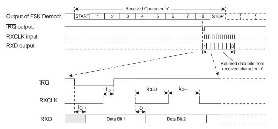
$t_D = Internal MX602 delay (max 1\mu S); t_{CLO} = RXCLK low time (min 1\mu S); t_{CHI} = RXCLK high time (min 1\mu S)$
