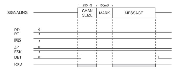
Figure 12: Bellcore System Signals (without ring)
