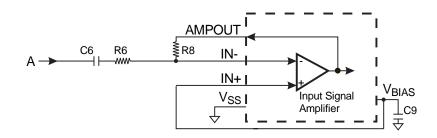
Figure 4: Input Signal Amplifier, unbalanced input configuration
